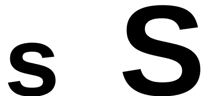
n / Example 7. The 48-point "S" has 1.78 times more area than the 36-point "S."
